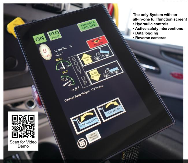
Allied's new complete truck monitoring control system for dump trucks actively monitors hydraulic and dump body operations as well as chassis operational data. This is a "whole truck" monitoring approach which allows for active intervention of unsafe equipment operation. Below are just a few things this system will do.
